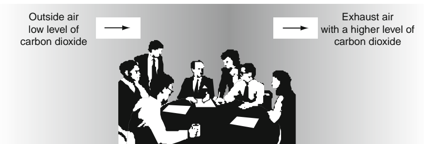
Figure 9-11 Ventilation Air Collecting CO 2 from Occupants
